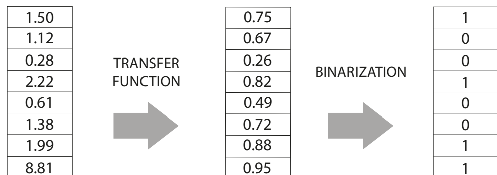
Figure 1. Two-step Binarization Scheme.
