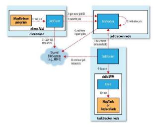
The **client** submits the MR job, the **jobtracker** coordinates the job run, the **tasktrackers** run the tasks that the job has been split into, and the **DFS** which is used for sharing job files.
