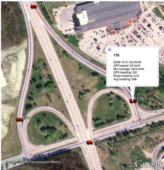
Figure 3: Illustration of the geo tracking process. The same vehicle appears at different points in time joined by the estimated trajectory.
